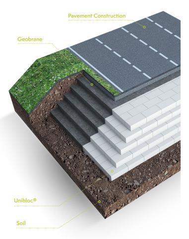
Unibloc® is manufactured to International Standard ASTM D6817 to ensure high quality Geofoam in lieu of no Australian standard in existence.
