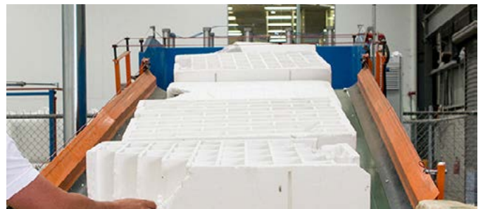
EPS offcuts being recycled at Unipod®.
